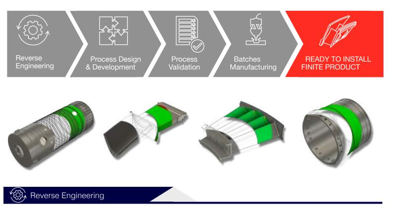
One or more samples are used to determine the Material and Shape of the component. For each stage of the production, complete manufacturing documentation, drawings and Quality Acceptance Protocols are drafted.
